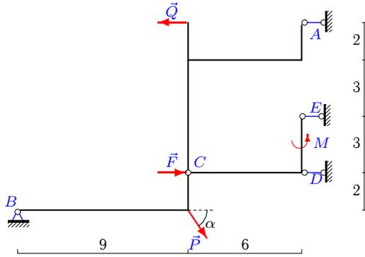
$P=6\text{кН}, Q=2\text{кН}, F=5\text{кН}, M = 3\text{кНм}, \alpha=60^\circ.$
