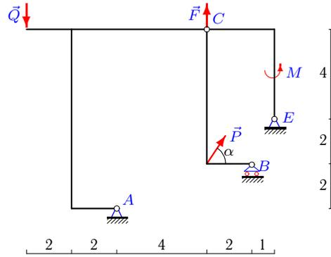
$$P=5\text{кН}, Q=1\text{кН}, F=2\text{кН}, M=6\text{кНм}, \alpha=60^\circ.$$
