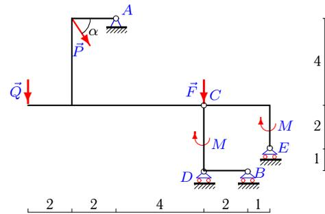
$P=1\text{кН}, Q=6\text{кН}, F=9\text{кН}, M = 6\text{кНм}, \alpha=60^\circ.$
