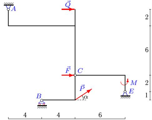
$$P=9\text{кН}, Q=6\text{кН}, F=2\text{кН}, M=5\text{кНм}, \alpha=30^\circ.$$
