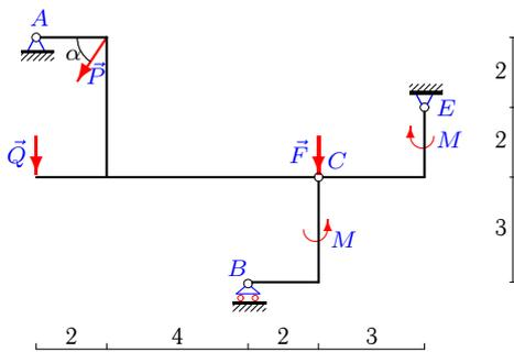
$P=5\text{кН}, Q=8\text{кН}, F=2\text{кН}, M = 3\text{кНм}, \alpha=60^\circ.$
