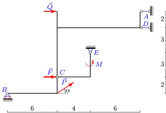
$P=3\text{кН}, Q=4\text{кН}, F=6\text{кН}, M=3\text{кНм}, \alpha=30^\circ.$
