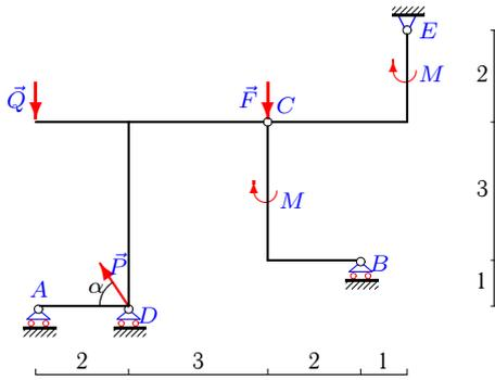
$P=3\text{кН}, Q=3\text{кН}, F=6\text{кН}, M=4\text{кНм}, \alpha=60^\circ.$
