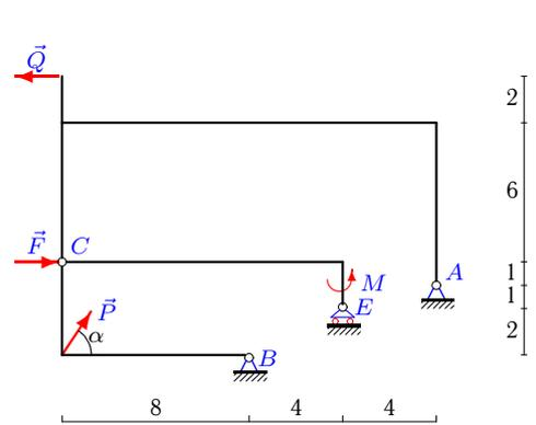
$$P=9\text{кН}, Q=7\text{кН}, F=3\text{кН}, M=6\text{кНм}, \alpha=60^\circ.$$
