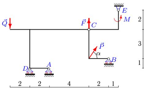
$P=9\text{кН}, Q=4\text{кН}, F=6\text{кН}, M = 4\text{кНм}, \alpha=60^\circ.$
