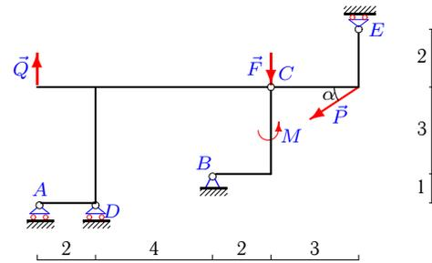
$P=5\text{кН}, Q=8\text{кН}, F=8\text{кН}, M = 3\text{кНм}, \alpha=30^\circ.$
