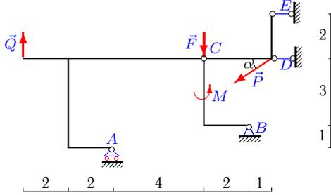
$$P=8\text{кН}, Q=8\text{кН}, F=5\text{кН}, M=4\text{кНм}, \alpha=30^\circ.$$
