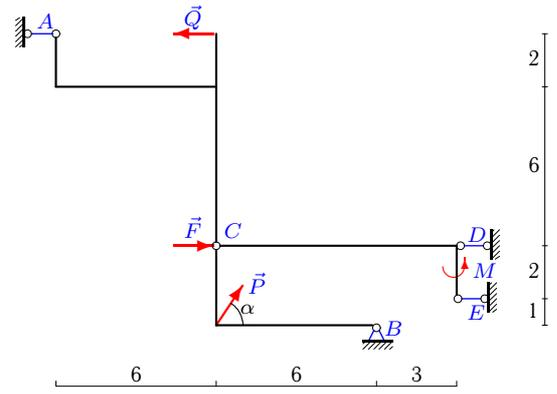
$P=3\text{кН}, Q=3\text{кН}, F=5\text{кН}, M = 6\text{кНм}, \alpha=60^\circ.$
