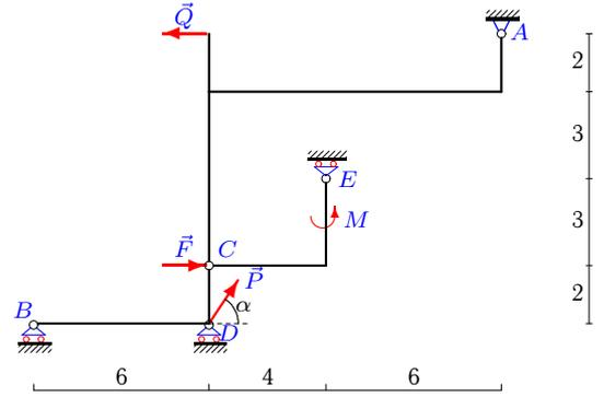
$P=6\text{кН}, Q=7\text{кН}, F=9\text{кН}, M = 3\text{кНм}, \alpha=60^\circ.$
