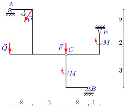
$P=1\text{кН}, Q=7\text{кН}, F=2\text{кН}, M = 4\text{кНм}, \alpha=60^\circ.$
