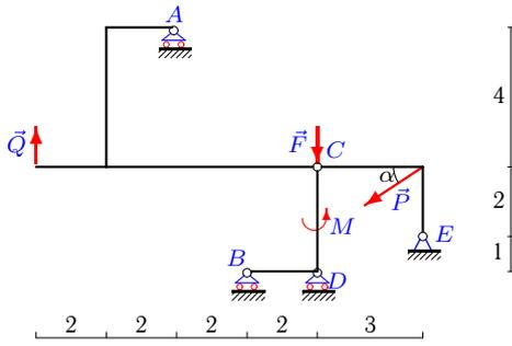
$P=5\text{кН}, Q=2\text{кН}, F=4\text{кН}, M = 5\text{кНм}, \alpha=30^\circ.$
