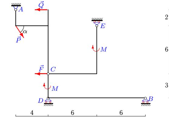
$P=8\text{кН}, Q=8\text{кН}, F=9\text{кН}, M = 4\text{кНм}, \alpha=60^\circ.$
