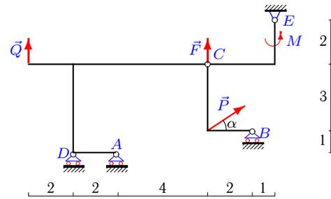
$P=9\text{кН}, Q=8\text{кН}, F=6\text{кН}, M=4\text{кНм}, \alpha=30^\circ.$
