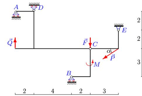
$P=4\text{кН}, Q=3\text{кН}, F=6\text{кН}, M = 3\text{кНм}, \alpha=30^\circ.$
