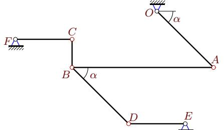
$$\omega_{OA_z} = -5\frac{1}{c}, \omega_{CF_z} = 10\frac{1}{c}, AB = 10, BC = 2, DE = 4, CF = 4, OA = BD = 4\sqrt{2}, \alpha = 45^\circ.$$
