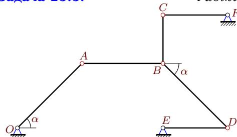
$$\omega_{CF_z} = \omega_{DE_z} = -15\frac{1}{2}, AB = 5, BC = 3, DE = 4, CF = 4, OA = BD = 4\sqrt{2}, \alpha = 45^\circ.$$
