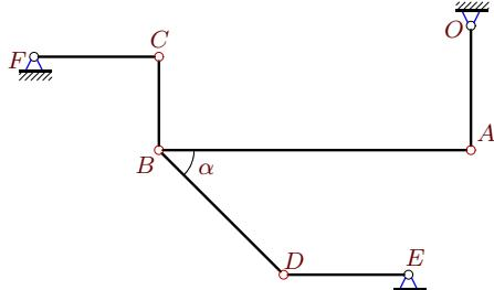
$$\omega_{CF_z} = -10\frac{1}{c}, \omega_{DE_z} = -5\frac{1}{c}, AB = 10, BC = 3, DE = 4, OA = 4, CF = 4, BD = 4\sqrt{2}, \alpha = 45^\circ.$$
