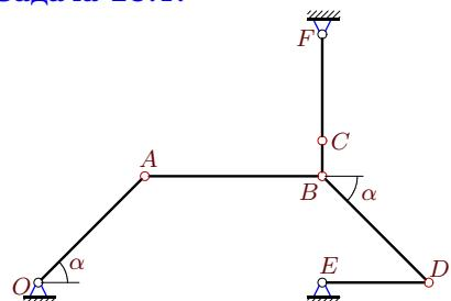
$$\omega_{CF_z} = -10\frac{1}{2}, \omega_{DE_z} = -5\frac{1}{2}, AB = 5, BC = 1, DE = 3, CF = 3, OA = BD = 3\sqrt{2}, \alpha = 45^\circ.$$
