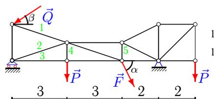
$$P = 50 \text{ кН}, Q = 60 \text{ кН}, F = 57 \text{ кН}, \\ \alpha = 35^\circ, \beta = 45^\circ.$$
