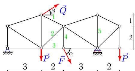
$$P = 20 \text{ кН}, Q = 90 \text{ кН}, F = 36 \text{ кН}, \\ \alpha = 65^\circ, \beta = 15^\circ.$$
