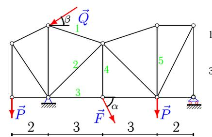
$$P = 60 \text{ кН}, Q = 40 \text{ кН}, F = 39 \text{ кН}, \\ \alpha = 40^\circ, \beta = 30^\circ.$$
