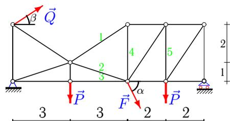
$$P = 80 \text{ кН}, Q = 40 \text{ кН}, F = 44 \text{ кН}, \\ \alpha = 50^\circ, \beta = 15^\circ.$$
