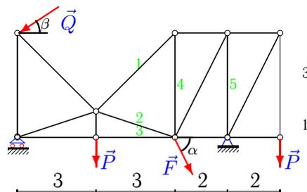
$$P = 20 \text{ кН}, Q = 30 \text{ кН}, F = 35 \text{ кН}, \\ \alpha = 65^\circ, \beta = 45^\circ.$$
