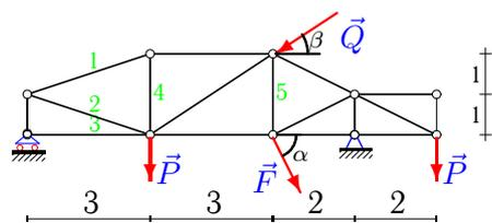
$$P = 40 \text{ кН}, Q = 90 \text{ кН}, F = 45 \text{ кН}, \\ \alpha = 75^\circ, \beta = 45^\circ.$$
