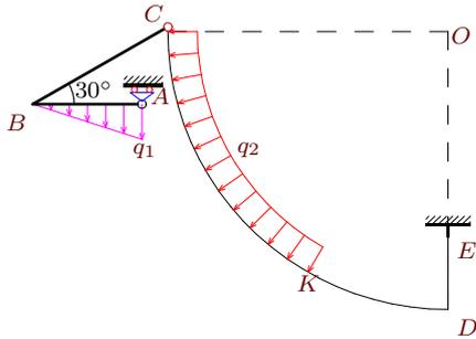
$$q_1 = 13 \text{ кН/м}, \quad R = 18 \text{ м},$$
