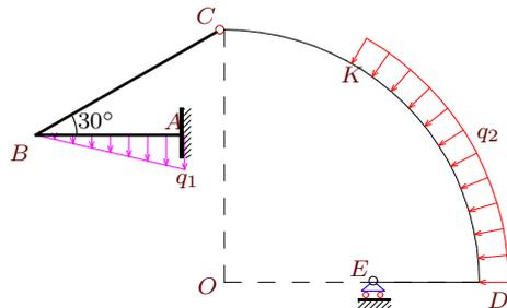
$$\begin{aligned} q_1 &= 12 \text{ кН/м}, & R &= 12 \text{ м}, \\ q_2 &= 7 \text{ кН/м}, & AB &= 7 \text{ м}, \\ & & BC &= 10 \text{ м}, & DK &= \pi R/3 \text{ м}, \\ & & DE &= 5 \text{ м}. \end{aligned}$$
