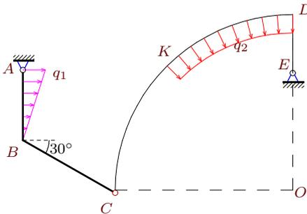
$$\begin{aligned} q_1 &= 13 \text{ кН/м}, & R &= 15 \text{ м}, \\ q_2 &= 8 \text{ кН/м}, & AB &= 6 \text{ м}, \\ & & BC &= 9 \text{ м}, & DK &= \pi R/4 \text{ м}, \\ & & DE &= 5 \text{ м}. \end{aligned}$$
