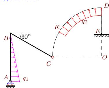
$$\begin{aligned} q_1 &= 11 \text{ кН/м}, & R &= 9 \text{ м}, \\ q_2 &= 10 \text{ кН/м}, & AB &= 9 \text{ м}, \\ BC &= 9 \text{ м}, & DK &= \pi R/3 \text{ м}, \\ DE &= 5 \text{ м}. \end{aligned}$$
