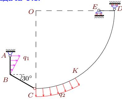
$$\begin{aligned} q_1 &= 10 \text{ кН/м}, & R &= 25 \text{ м}, \\ q_2 &= 5 \text{ кН/м}, & AB &= 6 \text{ м}, \\ & & BC &= 9 \text{ м}, & CK &= \pi R/6 \text{ м}, \\ & & DE &= 5 \text{ м}. \end{aligned}$$
