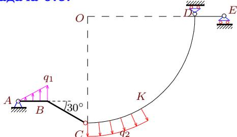
$$\begin{aligned} q_1 &= 11 \text{ кН/м}, & R &= 22 \text{ м}, \\ q_2 &= 6 \text{ кН/м}, & AB &= 6 \text{ м}, \\ BC &= 9 \text{ м}, & CK &= \pi R/6 \text{ м}, \\ DE &= 6 \text{ м}. \end{aligned}$$
