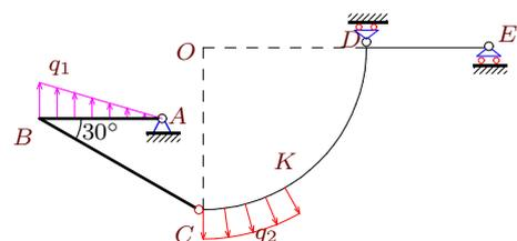
$$\begin{aligned} q_1 &= 15 \text{ кН/м}, & R &= 8 \text{ м}, \\ q_2 &= 6 \text{ кН/м}, & AB &= 6 \text{ м}, \\ BC &= 9 \text{ м}, & CK &= \pi R/6 \text{ м}, \\ DE &= 6 \text{ м}. \end{aligned}$$
