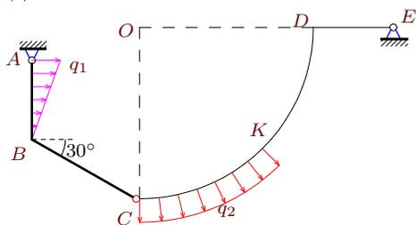
$$\begin{aligned} q_1 &= 13 \text{ кН/м}, & R &= 13 \text{ м}, \\ q_2 &= 8 \text{ кН/м}, & AB &= 6 \text{ м}, \\ BC &= 9 \text{ м}, & CK &= \pi R/4 \text{ м}, \\ DE &= 6 \text{ м}. \end{aligned}$$
