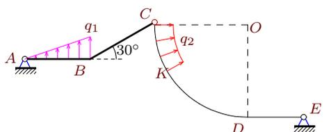
$$\begin{aligned} q_1 &= 16 \text{ кН/м}, & R &= 10 \text{ м}, \\ q_2 &= 4 \text{ кН/м}, & AB &= 7 \text{ м}, \\ BC &= 8 \text{ м}, & CK &= \pi R/6 \text{ м}, \\ DE &= 6 \text{ м}. \end{aligned}$$
