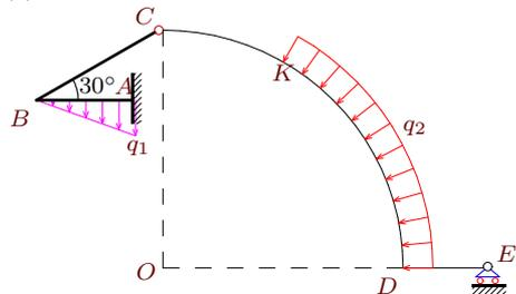
$$\begin{aligned} q_1 &= 15 \text{ кН/м}, & R &= 17 \text{ м}, \\ q_2 &= 7 \text{ кН/м}, & AB &= 7 \text{ м}, \\ & & BC &= 10 \text{ м}, & DK &= \pi R/3 \text{ м}, \\ & & DE &= 6 \text{ м}. \end{aligned}$$
