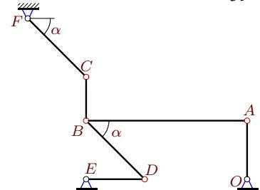
$$\omega_{CF_z} = 99\frac{1}{c}, \omega_{DE_z} = 33\frac{1}{c}, AB = 11, BC = 3, DE = 4, OA = 4, CF = BD = 4\sqrt{2}, \alpha = 45^\circ.$$
