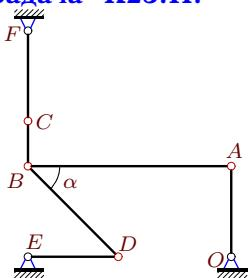
$$\omega_{OA_z} = 1\frac{1}{c}, \omega_{CF_z} = -2\frac{1}{c}, AB = 9, BC = 2, DE = 4, OA = 4, CF = 4, BD = 4\sqrt{2}, \alpha = 45^\circ.$$
