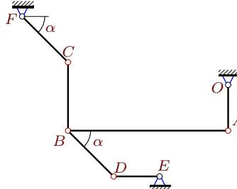
$$\omega_{OA_z} = -21\frac{1}{c}, \omega_{CF_z} = 63\frac{1}{c}, AB = 7, BC = 3, DE = 2, OA = 2, CF = BD = 2\sqrt{2}, \alpha = 45^\circ.$$
