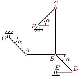
$$\omega_{CF_z} = -40\frac{1}{c}, \omega_{DE_z} = 40\frac{1}{c}, AB = 5, BC = 8, DE = 3, OA = CF = BD = 3\sqrt{2}, \alpha = 45^\circ.$$
