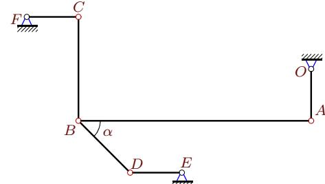
$$\omega_{CF_z} = 9\frac{1}{c}, \omega_{DE_z} = -9\frac{1}{c}, AB = 9, BC = 4, DE = 2, OA = 2, CF = 2, BD = 2\sqrt{2}, \alpha = 45^\circ.$$
