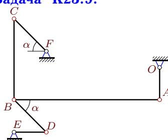
$$\omega_{CF_z} = -45\frac{1}{c}, \omega_{DE_z} = -15\frac{1}{c}, AB = 9, BC = 5, DE = 2, OA = 2, CF = BD = 2\sqrt{2}, \alpha = 45^\circ.$$
