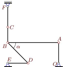
$$\omega_{CF_z} = 9\frac{1}{c}, \omega_{DE_z} = 3\frac{1}{c}, AB = 10, BC = 3, DE = 4, OA = 4, CF = 4, BD = 4\sqrt{2}, \alpha = 45^\circ.$$
