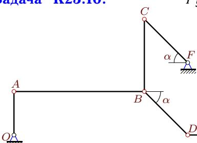
$$\omega_{OA_z} = 15\frac{1}{c}, \omega_{CF_z} = 30\frac{1}{c}, AB = 9, BC = 5, DE = 3, OA = 3, CF = BD = 3\sqrt{2}, \alpha = 45^\circ.$$
