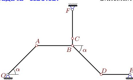
$$\omega_{OA_z} = 5\frac{1}{c}, \omega_{CF_z} = -10\frac{1}{c}, AB = 5, BC = 1, DE = 4, CF = 4, OA = BD = 4\sqrt{2}, \alpha = 45^\circ.$$
