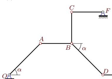
$$\omega_{CF_z} = -3\frac{1}{c}, \omega_{DE_z} = -1\frac{1}{c}, AB = 3, BC = 3, DE = 3, CF = 3, OA = BD = 3\sqrt{2}, \alpha = 45^\circ.$$
