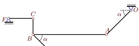
$$\omega_{CF_z} = 9\frac{1}{c}, \omega_{DE_z} = -3\frac{1}{c}, AB = 9, BC = 2, DE = 3, CF = 3, OA = BD = 3\sqrt{2}, \alpha = 45^\circ.$$
