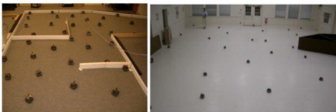
Figure 6: The iRobot swarm uniformly dispersed over a somewhat complex environment (left) and an open space (right).
