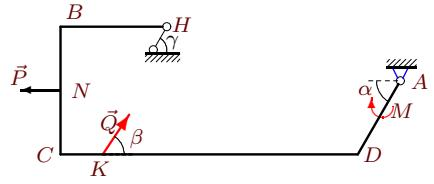
$$\begin{aligned}\rho &= 3 \text{ кН/м}, P = 9 \text{ кН}, Q = 31 \text{ кН}, \\ M &= 25 \text{ кНм}, \alpha = 60^\circ, \beta = 60^\circ, \gamma = 60^\circ, \\ HB &= 5 \text{ м}, BC = 6 \text{ м}, CD = 14 \text{ м}, \\ DA &= 4 \text{ м}, CK = 2 \text{ м}, CN = 3 \text{ м}.\end{aligned}$$
