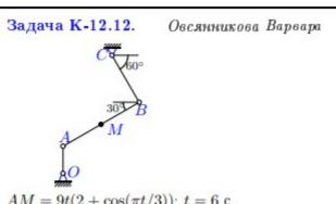
$$\begin{array}{l} AM = 9t(2+\cos(\pi t/3)); \; t = 6 \text{ c}, \\ \omega_{OA} = 1.3 \; \frac{1}{c}, \\ OA = 100, \; AB = 324, \; BC = 200 \end{array}$$
