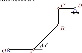
$$\begin{aligned}\omega_{OAz} &= -6, \quad \omega_{BCz} = -9, \\ \varepsilon_{OAz} &= -12, \quad \varepsilon_{BCz} = -273, \\ OA &= 3, \quad AB = 3\sqrt{2}, \quad BC = CD = 2.\end{aligned}$$
