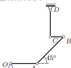
$$\begin{aligned}\omega_{OAz} &= -2, \quad \omega_{BCz} = -12, \\ \varepsilon_{OAz} &= -2, \quad \varepsilon_{BCz} = 32, \\ OA &= CD = 2, \quad AB = 2\sqrt{2}, \quad BC = 1.\end{aligned}$$
