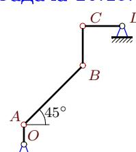
$$\begin{aligned}\omega_{OAz} &= -6, \quad \omega_{BCz} = 3, \\ \varepsilon_{OAz} &= 6, \quad \varepsilon_{BCz} = -24, \\ OA &= 1, \quad AB = 3\sqrt{2}, \quad BC = CD = 2.\end{aligned}$$
