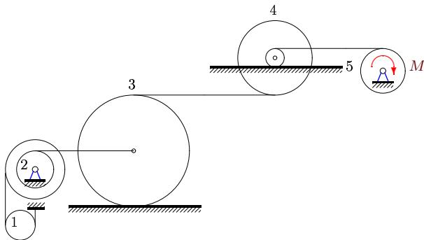
$$\begin{aligned} R_2 &= 4, r_2 = 2, \rho_2 = 2, \\ R_3 &= 6, \\ R_4 &= 4, r_4 = 1, \rho_4 = 3, \\ m_1 &= 8, m_2 = 16, \\ m_3 &= 14, m_4 = 54, \\ m_5 &= 90. \end{aligned}$$
