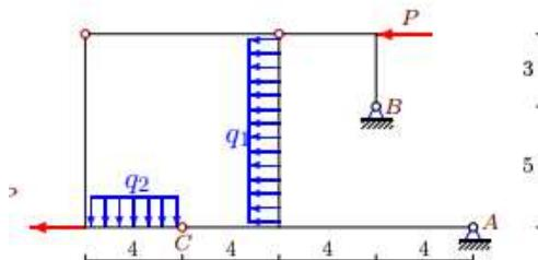
$$q_1 = 25 \text{ кН/м}, q_2 = 12 \text{ кН/м}, P = 18 \text{ кН}.$$
