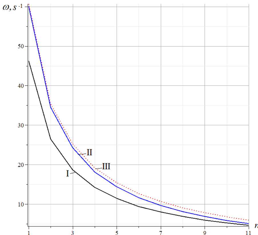
Fig. 3 - The first frequency of vibrations of the truss as a function of the number of panels.
