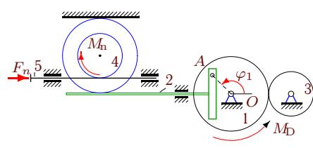
$$\begin{aligned}M_{Dz} &= M_0 - k\omega_{1z}, M_{nz} = -\mu\omega_{4z}, \\F_{nx} &= -\nu v_{5x}, \varphi_{1,0} = 1.3, \omega_{1z,0} = 0.4\frac{1}{c}, \\M_0 &= 12 \text{ Нм}, k = 14 \text{ Нмс}, \\&\nu = 30 \text{Нс/м}, \mu = 13 \text{ Нмс}, \\I_1 &= 15 \text{ кгм}^2, m_2 = 16 \text{ кг}, m_3 = 34 \text{ кг}, \\m_4 &= 26 \text{ кг}, R_1 = 37 \text{ см}, r_1 = 26 \text{ см}, \\R_3 &= 27 \text{ см}, R_4 = 20 \text{ см}, r_4 = 12 \text{ см}, i_4 = 15 \text{ см.}\end{aligned}$$
