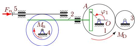
$$\begin{aligned} M_{Dz} &= M_0 - k\omega_{1z}, M_{nz} = -\mu\omega_{4z}, \\ F_{nx} &= -\nu v_{5x}, \varphi_{1,0} = 1.1, \omega_{1z,0} = 0.1\frac{1}{c}, \\ M_0 &= 10 \text{ Нм}, k = 11 \text{ Нмс}, \\ \nu &= 40 \text{ Гц/м}, \mu = 15 \text{ Нмс}, \\ I_1 &= 7 \text{ кгм}^2, m_2 = 14 \text{ кг}, m_3 = 32 \text{ кг}, \\ m_4 &= 24 \text{ кг}, R_1 = 34 \text{ см}, r_1 = 23 \text{ см}, \\ R_3 &= 24 \text{ см}, R_4 = 20 \text{ см}, r_4 = 12 \text{ см}, i_4 = 13 \text{ см}. \end{aligned}$$
