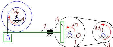
$$\begin{aligned}M_{Dz} &= M_0 - k\omega_{3z}, M_{nz} = -\mu\omega_{4z}, \\M_0 &= 11 \text{Нм}, k = 12 \text{Нмс}, \\&\varphi_{1,0} = 1.4, \omega_{1z,0} = 0.2\frac{1}{c}, \\&\mu = 12 \text{Нмс}, I_1 = 11 \text{ кгм}^2, \\m_2 &= 17 \text{ кг}, m_3 = 35 \text{ кг}, m_4 = 27 \text{ кг}, \\m_5 &= 6 \text{ кг}, R_1 = 35 \text{ см}, r_1 = 24 \text{ см}, \\R_3 &= 25 \text{ см}, R_4 = 20 \text{ см}, r_4 = 12 \text{ см}, i_4 = 16 \text{ см.}\end{aligned}$$
