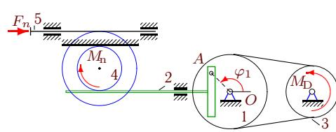
$$\begin{aligned}M_{Dz} &= M_0 - k\omega_{3z}, M_{nz} = -\mu\omega_{4z}, \\F_{nx} &= -\nu v_{5x}, \varphi_{1,0} = 1.3, \omega_{1z,0} = 0.3\frac{1}{c}, \\M_0 &= 10 \text{ Нм}, k = 13 \text{ Нмс}, \\&\nu = 8 \text{Нс/м}, \mu = 12 \text{ Нмс}, \\I_1 &= 9 \text{ кгм}^2, m_2 = 16 \text{ кг}, m_3 = 34 \text{ кг}, \\m_4 &= 26 \text{ кг}, R_1 = 36 \text{ см}, r_1 = 25 \text{ см}, \\R_3 &= 26 \text{ см}, R_4 = 20 \text{ см}, r_4 = 12 \text{ см}, i_4 = 15 \text{ см.}\end{aligned}$$
