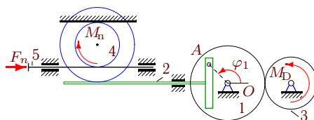
$$\begin{aligned} M_{Dz} &= M_0 - k\omega_{3z}, M_{nz} = -\mu\omega_{4z}, \\ F_{nx} &= -\nu v_{5x}, \varphi_{1,0} = 1.3, \omega_{1z,0} = 0.5\frac{1}{c}, \\ M_0 &= 9 \text{ Нм}, k = 15 \text{ Нмс}, \\ \nu &= 45 \text{ Гц/м}, \mu = 13 \text{ Нмс}, \\ I_1 &= 6 \text{ кгм}^2, m_2 = 16 \text{ кг}, m_3 = 34 \text{ кг}, \\ m_4 &= 26 \text{ кг}, R_1 = 38 \text{ см}, r_1 = 27 \text{ см}, \\ R_3 &= 28 \text{ см}, R_4 = 20 \text{ см}, r_4 = 12 \text{ см}, i_4 = 15 \text{ см}. \end{aligned}$$
