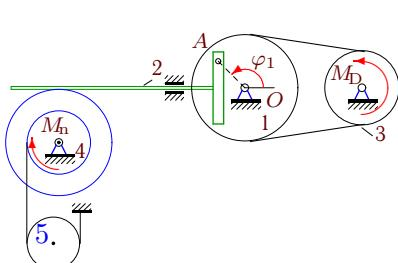
$$\begin{aligned} M_{Dz} &= M_0 - k\omega_{3z}, M_{nz} = -\mu\omega_{4z}, \\ M_0 &= 9 \text{ Нм}, k = 11 \text{ Нмс}, \\ \varphi_{1,0} &= 1.2, \omega_{1z,0} = 0.1\frac{1}{c}, \\ \mu &= 14 \text{ Нмс}, I_1 = 7 \text{ кгм}^2, \\ m_2 &= 15 \text{ кг}, m_3 = 33 \text{ кг}, m_4 = 25 \text{ кг}, \\ m_5 &= 4 \text{ кг}, R_1 = 34 \text{ см}, r_1 = 23 \text{ см}, \\ R_3 &= 24 \text{ см}, R_4 = 20 \text{ см}, r_4 = 12 \text{ см}, i_4 = 14 \text{ см}, \\ r_5 &= 11 \text{ см}. \end{aligned}$$
