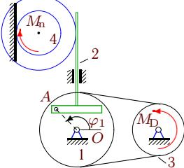
$$\begin{aligned} M_{Dz} &= M_0 - k\omega_{3z}, M_{nz} = -\mu\omega_{4z}, \\ \varphi_{1,0} &= 1.3, \omega_{1z,0} = 0.5\frac{1}{c}, \\ M_0 &= 10 \text{ Нм}, k = 15 \text{ Нмс}, \\ \mu &= 13 \text{ Нмс}, \\ I_1 &= 9 \text{ кгм}^2, m_2 = 16 \text{ кг}, m_3 = 34 \text{ кг}, \\ m_4 &= 26 \text{ кг}, R_1 = 38 \text{ см}, r_1 = 27 \text{ см}, \\ R_3 &= 28 \text{ см}, R_4 = 20 \text{ см}, r_4 = 12 \text{ см}, i_4 = 15 \text{ см}. \end{aligned}$$
