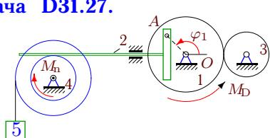
$$\begin{aligned} M_{Dz} &= M_0 - k\omega_{1z}, M_{nz} = -\mu\omega_{4z}, \\ M_0 &= 12 \text{ Нм}, k = 14 \text{ Нмс}, \\ \varphi_{1,0} &= 1.3, \omega_{1z,0} = 0.4\frac{1}{c}, \\ \mu &= 12 \text{ Нмс}, I_1 = 15 \text{ кгм}^2, \\ m_2 &= 16 \text{ кг}, m_3 = 34 \text{ кг}, m_4 = 26 \text{ кг}, \\ m_5 &= 6 \text{ кг}, R_1 = 37 \text{ см}, r_1 = 26 \text{ см}, \\ R_3 &= 27 \text{ см}, R_4 = 20 \text{ см}, r_4 = 12 \text{ см}, i_4 = 15 \text{ см}. \end{aligned}$$
