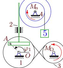
$$\begin{aligned}M_{Dz} &= M_0 - k\omega_{3z}, M_{nz} = -\mu\omega_{4z}, \\M_0 &= 9 \text{Нм}, k = 14 \text{Нмс}, \\&\varphi_{1,0} = 1.1, \omega_{1z,0} = 0.4\frac{1}{c}, \\&\mu = 15 \text{Нмс}, I_1 = 6 \text{ кгм}^2, \\m_2 &= 14 \text{ кг}, m_3 = 32 \text{ кг}, m_4 = 24 \text{ кг}, \\m_5 &= 4 \text{ кг}, R_1 = 37 \text{ см}, r_1 = 26 \text{ см}, \\R_3 &= 27 \text{ см}, R_4 = 20 \text{ см}, r_4 = 12 \text{ см}, i_4 = 13 \text{ см.}\end{aligned}$$
