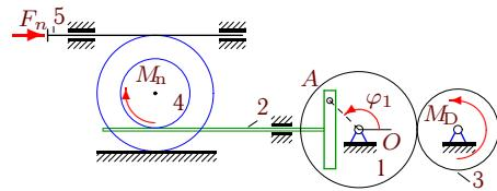
$$\begin{aligned}M_{Dz} &= M_0 - k\omega_{3z}, M_{nz} = -\mu\omega_{4z}, \\F_{nx} &= -\nu v_{5x}, \varphi_{1,0} = 1.5, \omega_{1z,0} = 0.5\frac{1}{c}, \\M_0 &= 11 \text{ Нм}, k = 15 \text{ Нмс}, \\&\nu = 10 \text{Нс/м}, \mu = 11 \text{ Нмс}, \\I_1 &= 8 \text{ кгм}^2, m_2 = 18 \text{ кг}, m_3 = 36 \text{ кг}, \\m_4 &= 28 \text{ кг}, R_1 = 38 \text{ см}, r_1 = 27 \text{ см}, \\R_3 &= 28 \text{ см}, R_4 = 20 \text{ см}, r_4 = 12 \text{ см}, i_4 = 17 \text{ см.}\end{aligned}$$
