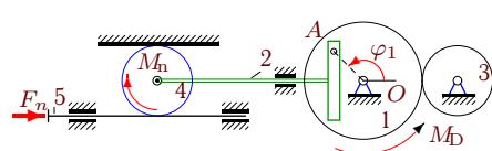
$$\begin{aligned}M_{Dz} &= M_0 - k\omega_{1z}, M_{nz} = -\mu\omega_{4z}, \\F_{nx} &= -\nu v_{5x}, \varphi_{1,0} = 1.4, \omega_{1z,0} = 0.4\frac{1}{c}, \\M_0 &= 13 \text{ Нм}, k = 14 \text{ Нмс}, \\&\nu = 40 \text{Нс/м}, \mu = 11 \text{ Нмс}, \\I_1 &= 19 \text{ кгм}^2, m_2 = 17 \text{ кг}, m_3 = 35 \text{ кг}, \\m_4 &= 27 \text{ кг}, R_1 = 37 \text{ см}, r_1 = 26 \text{ см}, \\R_3 &= 27 \text{ см}, R_4 = 12 \text{ см.}\end{aligned}$$
