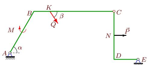
$$P = 6 \text{ kH}, Q = 2 \text{ kH}, M = 3 \text{ kHM}, \\ \rho = 1 \text{ kH/m}, \alpha = 60^\circ, \beta = 60^\circ, \\ AB = 6 \text{ m}, BC = 10 \text{ m}, CD = 6 \text{ m}, \\ DE = 3 \text{ m}, CN = 3 \text{ m}, BK = 2 \text{ m}.$$
