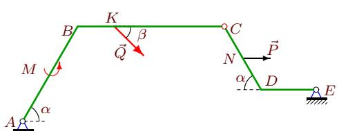
$$P = 5 \text{ kH}, Q = 6 \text{ kH}, M = 5 \text{ kHM}, \\ \rho = 1 \text{ kH/m}, \alpha = 60^\circ, \beta = 45^\circ, \\ AB = 6 \text{ m}, BC = 8 \text{ m}, CD = 4 \text{ m}, \\ DE = 3 \text{ m}, CN = 2 \text{ m}, BK = 2 \text{ m}.$$
