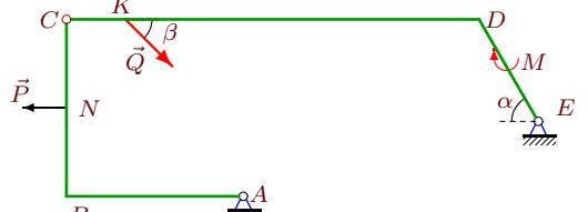
$$P = 5 \text{ kH}, Q = 9 \text{ kH}, M = 3 \text{ kHM}, \\ \rho = 1 \text{ kH/M}, \alpha = 60^\circ, \beta = 45^\circ, \\ AB = 6 \text{ m}, BC = 6 \text{ m}, CD = 14 \text{ m}, \\ DE = 4 \text{ m}, CN = 3 \text{ m}, CK = 2 \text{ m}.$$
