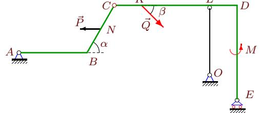
$$P = 6 \text{ kH}, Q = 1 \text{ kH}, M = 5 \text{ kHm}, \\ \rho = 2 \text{ kH/m}, \alpha = 60^\circ, \beta = 45^\circ, \\ AB = 5 \text{ m}, BC = 4 \text{ m}, CD = 9 \text{ m}, \\ DE = 7 \text{ m}, CN = 2 \text{ m}, CK = 2 \text{ m}, LD = 2 \text{ m}$$
