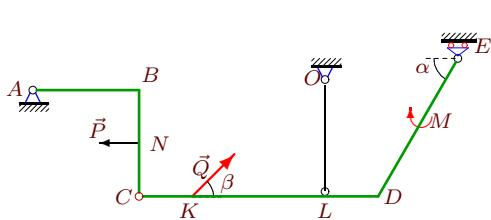
$$P = 6 \text{ kH}, Q = 7 \text{ kH}, M = 6 \text{ kHM}, \\ \rho = 2 \text{ kH/m}, \alpha = 60^\circ, \beta = 45^\circ, \\ AB = 4 \text{ m}, BC = 4 \text{ m}, CD = 9 \text{ m}, \\ DE = 6 \text{ m}, CN = 2 \text{ m}, CK = 2 \text{ m}, LD = 2 \text{ m}$$
