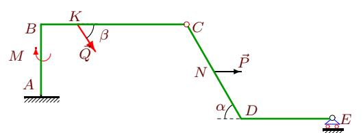
$$P = 8 \text{ kH}, Q = 8 \text{ kH}, M = 9 \text{ kHM}, \\ \rho = 3 \text{ kH/m}, \alpha = 60^\circ, \beta = 60^\circ, \\ AB = 4 \text{ m}, BC = 8 \text{ m}, CD = 6 \text{ m}, \\ DE = 5 \text{ m}, CN = 3 \text{ m}, BK = 2 \text{ m}.$$
