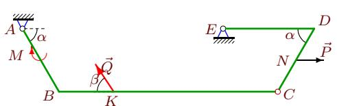
$$\begin{aligned} P &= 7 \text{ kH}, Q = 4 \text{ kH}, M = 3 \text{ kHM}, \\ \rho &= 1 \text{ kH/m}, \alpha = 60^\circ, \beta = 75^\circ, \\ AB &= 4 \text{ m}, BC = 12 \text{ m}, CD = 4 \text{ m}, \\ DE &= 5 \text{ m}, CN = 2 \text{ m}, BK = 3 \text{ m}. \end{aligned}$$
