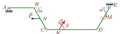
$$P = 7 \text{ kH}, Q = 6 \text{ kH}, M = 9 \text{ kHM}, \\ \rho = 1 \text{ kH/M}, \alpha = 60^\circ, \beta = 75^\circ, \\ AB = 4 \text{ m}, BC = 4 \text{ m}, CD = 8 \text{ m}, \\ DE = 4 \text{ m}, CN = 2 \text{ m}, CK = 2 \text{ m}.$$
