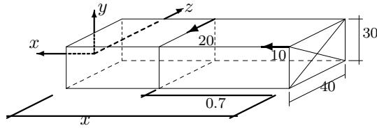
$N = 10\text{kH}$ ;  $Q_y = 0$ ;  $Q_z = -20\text{kH}$ ;  $M_x = +20 \cdot 0.15 = 3\text{kNm}$ ;  $M_y(0.7) = +10 \cdot 0.2 = 2\text{kNm}$ ;  $M_y(1.2) = +10 \cdot 0.2 + 20 \cdot 0.5 = 12\text{kNm}$ ;  $M_z = +10 \cdot 0.15 = 1.5\text{kNm}$ ;
