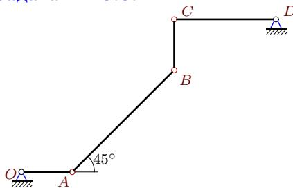
$$\begin{aligned}\omega_{OAz} &= \omega_{BCz} = -2 \text{ рад/с}, \\ \varepsilon_{OAz} &= -6 \text{ рад/с}^2, \quad \varepsilon_{CDz} = -2 \text{ рад/с}^2, \\ OA &= 1, \quad AB = 2\sqrt{2}, \quad BC = 1, \quad CD = 2.\end{aligned}$$
