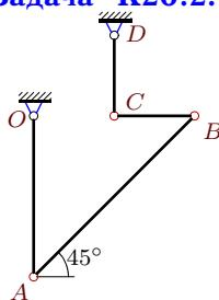
$$\begin{aligned}\omega_{OAz} &= -2 \text{ рад/с}, \quad \omega_{CDz} = 2 \text{ рад/с}, \\ \varepsilon_{OAz} &= -2 \text{ рад/с}^2, \quad \varepsilon_{BCz} = 2 \text{ рад/с}^2, \\ OA &= 2, \quad AB = 2\sqrt{2}, \quad BC = CD = 1.\end{aligned}$$
