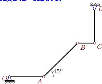
$$\begin{aligned}\omega_{OAz} &= 2 \text{ рад/с}, \quad \omega_{BCz} = 4 \text{ рад/с}, \\ \varepsilon_{OAz} &= 2 \text{ рад/с}^2, \quad \varepsilon_{BCz} = 116 \text{ рад/с}^2, \\ OA &= 2, \quad AB = 2\sqrt{2}, \quad BC = 1, \quad CD = 2.\end{aligned}$$
