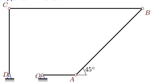
$$\begin{aligned}\omega_{OAz} &= -8 \text{ рад/с}, \quad \omega_{CDz} = 0, \\ \varepsilon_{BCz} &= -20 \text{ рад/с}^2, \quad \varepsilon_{CDz} = -16 \text{ рад/с}^2, \\ OA &= 1, \quad AB = 2\sqrt{2}, \quad BC = 4, \quad CD = 2.\end{aligned}$$
