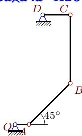
$$\begin{aligned}\omega_{OAz} &= -15 \text{ рад/с}, \quad \omega_{BCz} = 9 \text{ рад/с}, \\ \varepsilon_{BCz} &= -45 \text{ рад/с}^2, \quad \varepsilon_{CDz} = 15 \text{ рад/с}^2, \\ OA &= 1, \quad AB = 3\sqrt{2}, \quad BC = 5, \quad CD = 2.\end{aligned}$$
