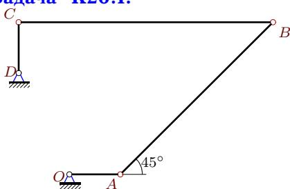
$$\begin{aligned}\omega_{OAz} &= -15 \text{ рад/с}, \quad \omega_{CDz} = 0, \\ \varepsilon_{OAz} &= -15 \text{ рад/с}^2, \quad \varepsilon_{BCz} = -42 \text{ рад/с}^2, \\ OA &= 1, \quad AB = 3\sqrt{2}, \quad BC = 5, \quad CD = 1.\end{aligned}$$
