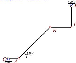
$$\begin{aligned} \omega_{BCz} &= -3 \text{ рад/с}, \quad \omega_{CDz} = 0, \\ \varepsilon_{OAz} &= 0, \quad \varepsilon_{BCz} = 39 \text{ рад/с}^2, \\ OA &= 1, \quad AB = 3\sqrt{2}, \quad BC = CD = 2. \end{aligned}$$
