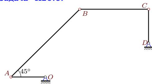
$$\begin{aligned} \omega_{BCz} &= 2 \text{ рад/с}, \quad \omega_{CDz} = 0, \\ \varepsilon_{OAz} &= \varepsilon_{BCz} = -4 \text{ рад/с}^2, \\ OA &= 1, \quad AB = 2\sqrt{2}, \quad BC = 2, \quad CD = 1. \end{aligned}$$
