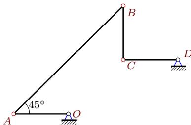
$$\begin{aligned} \omega_{OAz} &= \omega_{BCz} = 2 \text{ рад/с}, \\ \varepsilon_{OAz} &= -2 \text{ рад/с}^2, \quad \varepsilon_{BCz} = -8 \text{ рад/с}^2, \\ OA &= 1, \quad AB = 2\sqrt{2}, \quad BC = CD = 1. \end{aligned}$$
