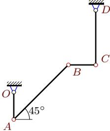
$$\begin{aligned} \omega_{BCz} &= -2 \text{ рад/с}, \quad \omega_{CDz} = 0, \\ \varepsilon_{BCz} &= \varepsilon_{CDz} = 2 \text{ рад/с}^2, \\ OA &= 1, \quad AB = 2\sqrt{2}, \quad BC = 1, \quad CD = 2. \end{aligned}$$
