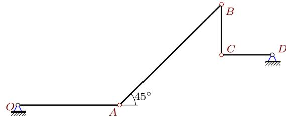
$$\begin{aligned} \omega_{BCz} &= -6 \text{ рад/с}, \quad \omega_{CDz} = 2 \text{ рад/с}, \\ \varepsilon_{BCz} &= \varepsilon_{CDz} = 4 \text{ рад/с}^2, \\ OA &= 2, \quad AB = 2\sqrt{2}, \quad BC = CD = 1. \end{aligned}$$
