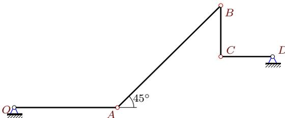
$$\begin{aligned} \omega_{BCz} &= -6 \text{ рад/с}, \quad \omega_{CDz} = 2 \text{ рад/с}, \\ \varepsilon_{OAz} &= 2 \text{ рад/с}^2, \quad \varepsilon_{BCz} = 8 \text{ рад/с}^2, \\ OA &= 2, \quad AB = 2\sqrt{2}, \quad BC = CD = 1. \end{aligned}$$
