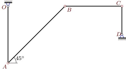
$$\begin{aligned}\omega_{OAz} &= 4 \text{ рад/с}, \omega_{BCz} = -4 \text{ рад/с}, \\ \varepsilon_{BCz} &= 26 \text{ рад/с}^2, \varepsilon_{CDz} = 4 \text{ рад/с}^2, \\ OA &= 2, AB = 2\sqrt{2}, BC = 2, CD = 1.\end{aligned}$$
