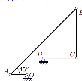
$$\begin{aligned}\omega_{OAz} &= 12 \text{ рад/с}, \omega_{BCz} = 20 \text{ рад/с}, \\ \varepsilon_{BCz} &= -220 \text{ рад/с}^2, \varepsilon_{CDz} = 24 \text{ рад/с}^2, \\ OA &= 1, AB = 4\sqrt{2}, BC = 3, CD = 2.\end{aligned}$$
