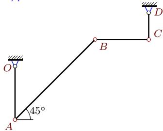
$$\begin{aligned}\omega_{OAz} &= 6 \text{ рад/с}, \omega_{CDz} = -6 \text{ рад/с}, \\ \varepsilon_{OAz} &= 6 \text{ рад/с}^2, \varepsilon_{BCz} = 171 \text{ рад/с}^2, \\ OA &= 2, AB = 3\sqrt{2}, BC = 2, CD = 1.\end{aligned}$$
