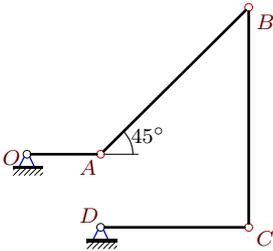
$$\begin{aligned} \omega_{OAz} &= \omega_{BCz} = 6 \text{ рад/с}, \\ \varepsilon_{OAz} &= 0, \quad \varepsilon_{BCz} = -4 \text{ рад/с}^2, \\ OA &= 1, \quad AB = 2\sqrt{2}, \quad BC = 3, \quad CD = 2. \end{aligned}$$
