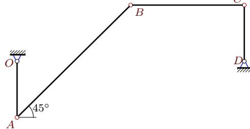
$$\begin{aligned} \omega_{BCz} &= -2 \text{ рад/с}, \quad \omega_{CDz} = 0, \\ \varepsilon_{BCz} &= 0, \quad \varepsilon_{CDz} = 8 \text{ рад/с}^2, \\ OA &= 1, \quad AB = 2\sqrt{2}, \quad BC = 2, \quad CD = 1. \end{aligned}$$
