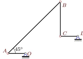
$$\begin{aligned} \omega_{OAz} &= 6 \text{ рад/с}, \quad \omega_{BCz} = 3 \text{ рад/с}, \\ \varepsilon_{OAz} &= -6 \text{ рад/с}^2, \quad \varepsilon_{BCz} = -24 \text{ рад/с}^2, \\ OA &= 1, \quad AB = 3\sqrt{2}, \quad BC = 2, \quad CD = 1. \end{aligned}$$
