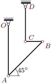
$$\begin{aligned} \omega_{BCz} &= 2 \text{ рад/с}, \quad \omega_{CDz} = -4 \text{ рад/с}, \\ \varepsilon_{OAz} &= -4 \text{ рад/с}^2, \quad \varepsilon_{BCz} = -28 \text{ рад/с}^2, \\ OA &= 3, \quad AB = 2\sqrt{2}, \quad BC = 1, \quad CD = 2. \end{aligned}$$
