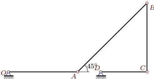
$$\begin{aligned} \omega_{BCz} &= -9 \text{ рад/с}, \quad \omega_{CDz} = 0, \\ \varepsilon_{OAz} &= 18 \text{ рад/с}^2, \quad \varepsilon_{CDz} = 9 \text{ рад/с}^2, \\ OA &= 3, \quad AB = 3\sqrt{2}, \quad BC = 3, \quad CD = 2. \end{aligned}$$
