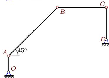
$$\begin{aligned} \omega_{OAz} &= 9 \text{ рад/с}, \quad \omega_{BCz} = 3 \text{ рад/с}, \\ \varepsilon_{OAz} &= -9 \text{ рад/с}^2, \quad \varepsilon_{BCz} = 45 \text{ рад/с}^2, \\ OA &= 1, \quad AB = 3\sqrt{2}, \quad BC = 3, \quad CD = 2. \end{aligned}$$
