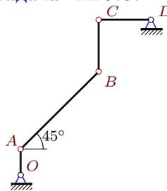
$$\begin{aligned} \omega_{OAz} &= -6 \text{ рад/с}, \quad \omega_{BCz} = 3 \text{ рад/с}, \\ \varepsilon_{BCz} &= -24 \text{ рад/с}^2, \quad \varepsilon_{CDz} = 6 \text{ рад/с}^2, \\ OA &= 1, \quad AB = 3\sqrt{2}, \quad BC = CD = 2. \end{aligned}$$
