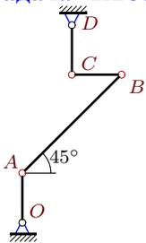
$$\begin{aligned} \omega_{OAz} &= -2 \text{ рад/с}, \quad \omega_{BCz} = 4 \text{ рад/с}, \\ \varepsilon_{BCz} &= -12 \text{ рад/с}^2, \quad \varepsilon_{CDz} = 2 \text{ рад/с}^2, \\ OA &= 1, \quad AB = 2\sqrt{2}, \quad BC = CD = 1. \end{aligned}$$
