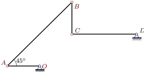
$$\begin{aligned} \omega_{OAz} &= 2 \text{ рад/с}, \quad \omega_{CDz} = 0, \\ \varepsilon_{BCz} &= -14 \text{ рад/с}^2, \quad \varepsilon_{CDz} = 4 \text{ рад/с}^2, \\ OA &= 1, \quad AB = 2\sqrt{2}, \quad BC = 1, \quad CD = 2. \end{aligned}$$
