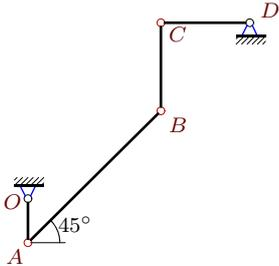
$$\begin{aligned} \omega_{BCz} &= -3 \text{ рад/с}, \quad \omega_{CDz} = 0, \\ \varepsilon_{BCz} &= 3 \text{ рад/с}^2, \quad \varepsilon_{CDz} = -6 \text{ рад/с}^2, \\ OA &= 1, \quad AB = 3\sqrt{2}, \quad BC = CD = 2. \end{aligned}$$
