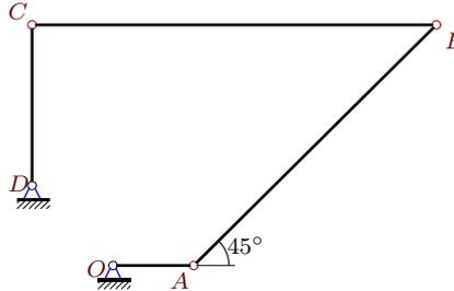
$$\begin{aligned} \omega_{OAz} &= -15 \text{ рад/с}, \quad \omega_{BCz} = -3 \text{ рад/с}, \\ \varepsilon_{OAz} &= 15 \text{ рад/с}^2, \quad \varepsilon_{BCz} = -45 \text{ рад/с}^2, \\ OA &= 1, \quad AB = 3\sqrt{2}, \quad BC = 5, \quad CD = 2. \end{aligned}$$
