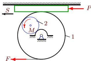
$m_1 = 4 \text{ кг}, m_2 = 48 \text{ кг}, R_2 = 30 \text{ см}, R_1 = \rho_1, M = 24 \text{ Нм}, F = 150 \text{ Н}, P = 215 \text{ Н}, S = 44 \text{ см}.$
