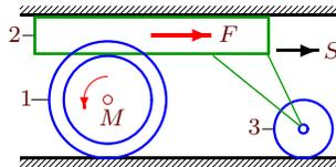
$m_1 = 4.9 \text{ кг}, m_2 = 3 \text{ кг}, m_3 = 10 \text{ кг}, R_1 = 4 \text{ см}, r_1 = 3 \text{ см}, \rho_1 = 4 \text{ см}, M = 6.3 \text{ Нм}, F = 94 \text{ Н}, S = 42.4 \text{ см}.$
