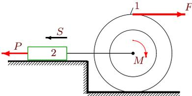
$m_1 = 25 \text{ кг}, m_2 = 4 \text{ кг}, F = 20 \text{ Н}, P = 173 \text{ Н}, M = 5 \text{ Нм}, r = 3 \text{ см}, R = 5 \text{ см}, \rho = 2 \text{ см}, S = 128 \text{ см}.$
