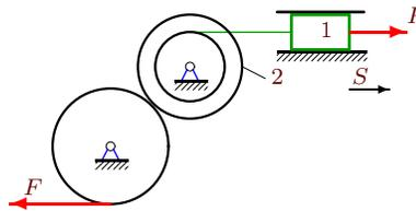
$m_1 = 1 \text{ кг}$ ,  $m_2 = 12 \text{ кг}$ ,  $R_2 = 30 \text{ см}$ ,  $r_2 = 20 \text{ см}$ ,  $\rho_2 = 30 \text{ см}$ ,  $F = 4 \text{ Н}$ ,  $P = 70 \text{ Н}$ ,
