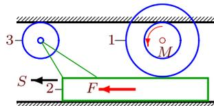
$m_1 = 3.6 \text{ кг}, m_2 = 2 \text{ кг}, m_3 = 6 \text{ кг}, R_1 = 4 \text{ см}, r_1 = 2 \text{ см}, \rho_1 = 3 \text{ см}, M = 5.4 \text{ Нм}, F = 94 \text{ Н}, S = 24.6 \text{ см}.$
