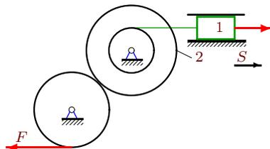
$m_1 = 1 \text{ кг}$ ,  $m_2 = 12 \text{ кг}$ ,  $R_2 = 40 \text{ см}$ ,  $r_2 = 20 \text{ см}$ ,  $\rho_2 = 30 \text{ см}$ ,  $F = 4 \text{ Н}$ ,  $P = 72 \text{ Н}$ ,
