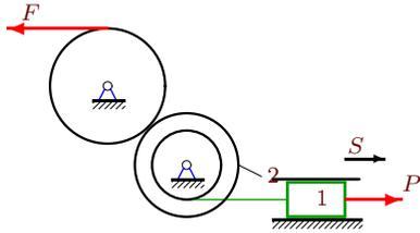
$m_1 = 2 \text{ кг}, m_2 = 20 \text{ кг}, R_2 = 30 \text{ см}, r_2 = 20 \text{ см}, \rho_2 = 20 \text{ см}, F = 6 \text{ Н}, P = 45 \text{ Н}, S = 44 \text{ см}.$
