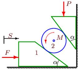
$m_1 = 0.1 \text{ кг}, m_2 = 0.49 \text{ кг}, F = 2 \text{ Н}, P = 43 \text{ Н}, M = 28 \text{ Нм}, R = 0.4 \text{ м}, S = 20.25 \text{ см}, \cos \alpha = 0.8.$
