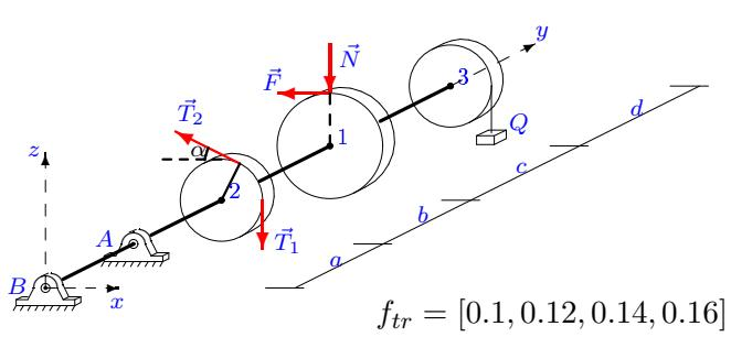
$$\begin{aligned}F &= fN, T_1 = 40, \\T_2 &= 21, P_1 = 36, \\P_2 = 30, P_3 &= 34, \\Q &= 26, G = 20, \\\alpha &= 60^\circ, R_1 = 18, \\R_2 = 12, R_3 &= 13, \\a = 22, b = 27, \\c = 30, d = 23.\end{aligned}$$
