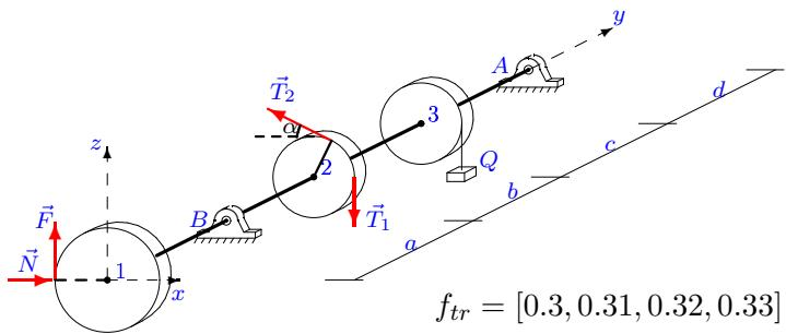
$$\begin{aligned}F &= fN, T_1 = 60, \\T_2 &= 118, P_1 = 32, \\P_2 = 20, P_3 &= 28, \\Q &= 14, G = 30, \\\alpha &= 45^\circ, R_1 = 20, \\R_2 = 10, R_3 &= 12, \\a = 24, b = 26, \\c = 28, d = 26.\end{aligned}$$
