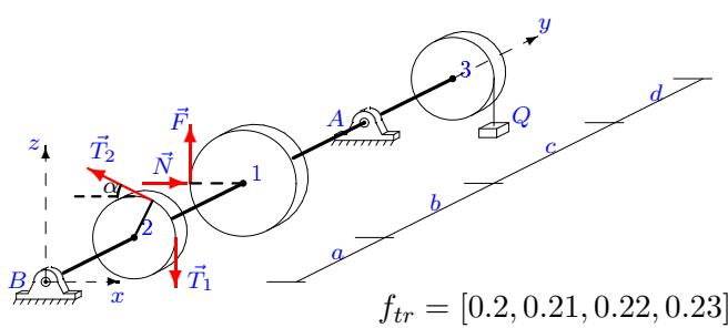
$$F = fN, T_1 = 40, \\ T_2 = 77, P_1 = 28, \\ P_2 = 20, P_3 = 24, \\ Q = 18, G = 20, \\ \alpha = 45^\circ, R_1 = 20, \\ R_2 = 10, R_3 = 11, \\ a = 22, b = 25, \\ c = 27, d = 24.$$
