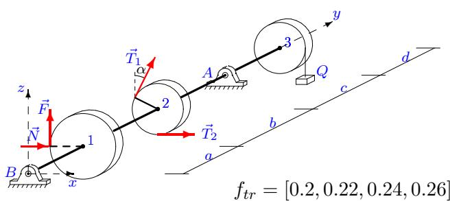
$$F = fN, T_1 = 40, \\ T_2 = 77, P_1 = 32, \\ P_2 = 20, P_3 = 24, \\ Q = 18, G = 20, \\ \alpha = 45^\circ, R_1 = 28, \\ R_2 = 10, R_3 = 11, \\ a = 22, b = 25, \\ c = 27, d = 26.$$
