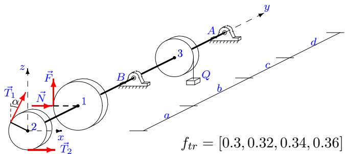
$$\begin{aligned}F &= fN, T_1 = 50, \\T_2 &= 98, P_1 = 34, \\P_2 &= 20, P_3 = 28, \\Q &= 14, G = 25, \\\alpha &= 45^\circ, R_1 = 24, \\R_2 &= 10, R_3 = 12, \\a &= 24, b = 26, \\c &= 28, d = 27.\end{aligned}$$
