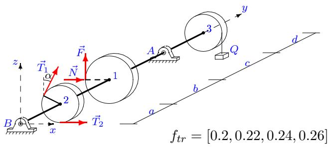
$$\begin{aligned}F &= fN, T_1 = 40, \\T_2 &= 78, P_1 = 40, \\P_2 &= 30, P_3 = 34, \\Q &= 14, G = 20, \\\alpha &= 60^\circ, R_1 = 26, \\R_2 &= 12, R_3 = 13, \\a &= 22, b = 24, \\c &= 27, d = 25.\end{aligned}$$
