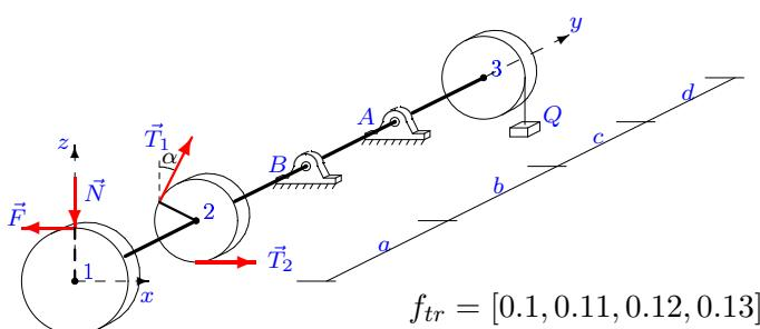
$$F = fN, T_1 = 60, \\ T_2 = 31, P_1 = 30, \\ P_2 = 20, P_3 = 24, \\ Q = 26, G = 30, \\ \alpha = 45^\circ, R_1 = 24, \\ R_2 = 10, R_3 = 11, \\ a = 22, b = 27, \\ c = 29, d = 25.$$
