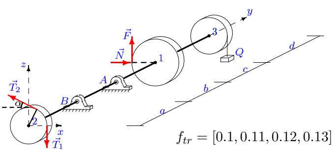
$$\begin{aligned}F &= fN, T_1 = 50, \\T_2 &= 96, P_1 = 18, \\P_2 = 10, P_3 &= 14, \\Q &= 22, G = 25, \\\alpha &= 30^\circ, R_1 = 18, \\R_2 = 8, R_3 &= 9, \\a = 22, b = 26, \\c = 27, d = 24.\end{aligned}$$
