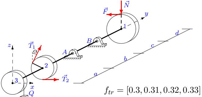
$$\begin{aligned}F &= fN, T_1 = 70, \\T_2 &= 38, P_1 = 24, \\P_2 &= 10, P_3 = 18, \\Q &= 10, G = 35, \\\alpha &= 30^\circ, R_1 = 22, \\R_2 &= 8, R_3 = 10, \\a &= 24, b = 25, \\c &= 26, d = 27.\end{aligned}$$
