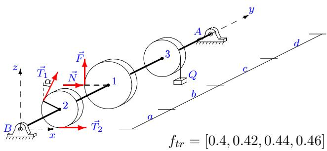
$$\begin{aligned}F &= fN, T_1 = 40, \\T_2 &= 76, P_1 = 44, \\P_2 = 30, P_3 &= 38, \\Q &= 22, G = 20, \\\alpha &= 60^\circ, R_1 = 26, \\R_2 = 12, R_3 &= 14, \\a = 24, b = 28, \\c = 31, d = 27.\end{aligned}$$
