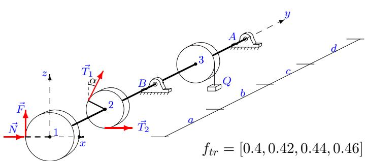
$$\begin{aligned}F &= fN, T_1 = 60, \\T_2 &= 116, P_1 = 34, \\P_2 &= 20, P_3 = 28, \\Q &= 22, G = 30, \\\alpha &= 45^\circ, R_1 = 24, \\R_2 &= 10, R_3 = 12, \\a &= 24, b = 28, \\c &= 30, d = 27.\end{aligned}$$
