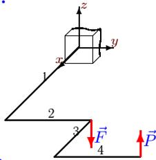
$$\begin{aligned} l_1 &= 2 \text{ м}, \\ l_2 &= 2 \text{ м}, \\ l_3 &= 1 \text{ м}, \\ l_4 &= 2 \text{ м}, \\ P &= 1 \text{ кН}, \\ F &= 2 \text{ кН}. \end{aligned}$$
