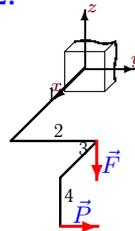
$$\begin{aligned} l_1 &= 2 \text{ м}, \\ l_2 &= 2 \text{ м}, \\ l_3 &= 1 \text{ м}, \\ l_4 &= 1 \text{ м}, \\ P &= 3 \text{ кН}, \\ F &= 2 \text{ кН}. \end{aligned}$$
