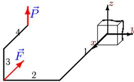
$$\begin{aligned} l_1 &= 2 \text{ м}, \\ l_2 &= 2 \text{ м}, \\ l_3 &= 1 \text{ м}, \\ l_4 &= 1 \text{ м}, \\ P &= 2 \text{ кН}, \\ F &= 3 \text{ кН}. \end{aligned}$$
